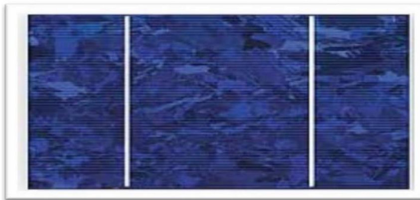
Figure II.18 : Cellule Si polycristallin(Mc-Si)
