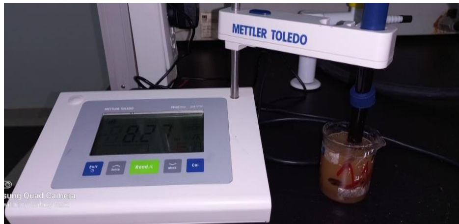
Figure 10: Preparation and Measurement of the pH of a soil sample using a pH meter
