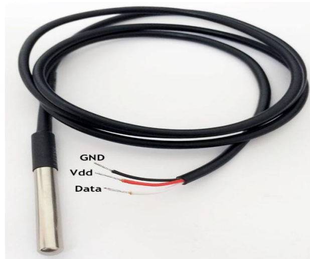
Figure III. 8: DS18B20 Arduino Temperature sensor. [86]
