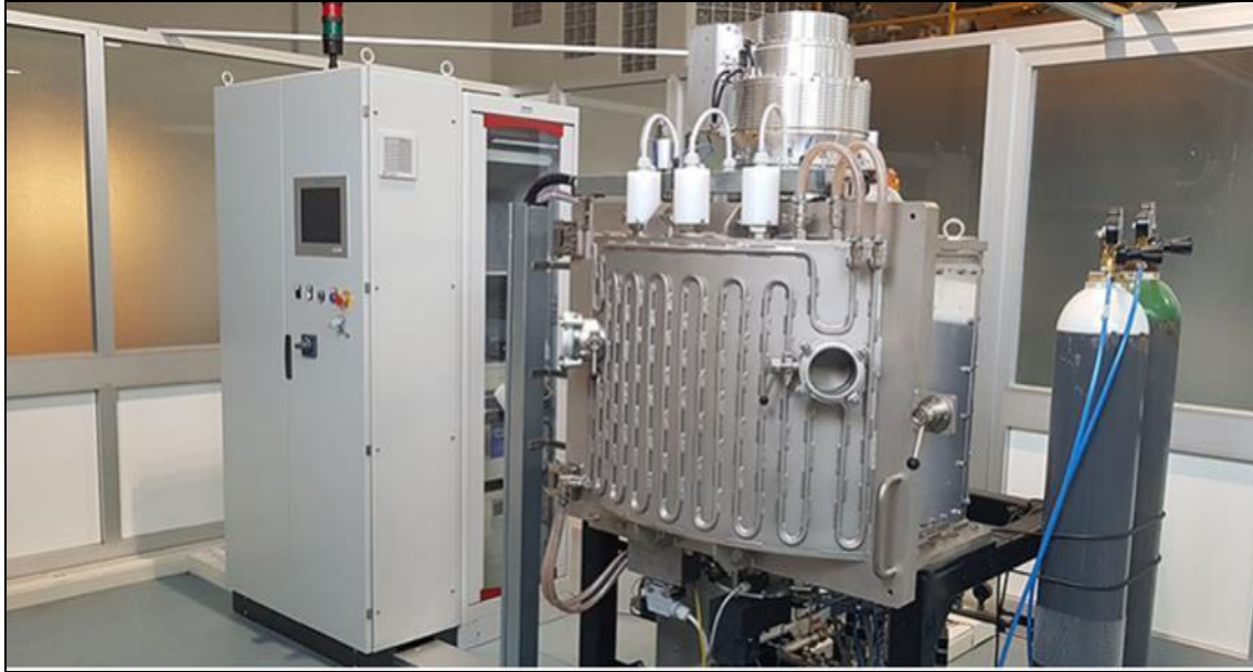
Figure II.3 Vacuum chambers for the deposition of thin film.
