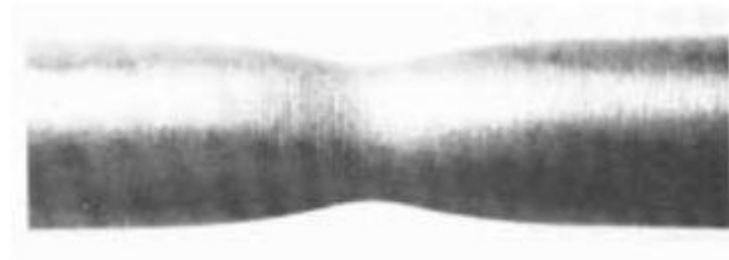
Figure I.7: Necking in a tensile specimen.
