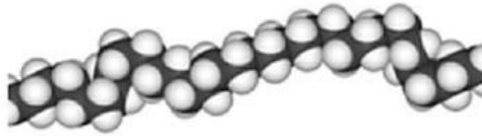
Figure I.2: Representative diagram of polyethylene.
