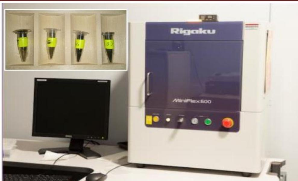
Figure III. 6: Diffractomètre Rigaku miniflex 600 X-ray.
