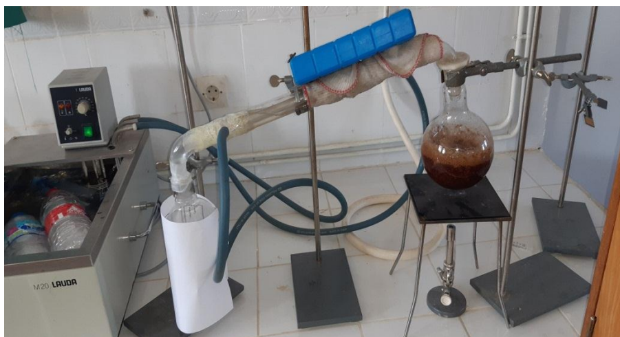
Figure 16 : Montage de l'hydro distillation (original)
