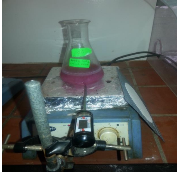
Figure III.5 : Séchage de solution \text{SnO}_2/\text{ZnCO}_2\text{O}_4
