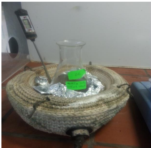
Figure III.6 : Séchage de \text{SnO}_2/\text{ZnCO}_2\text{O}_4
