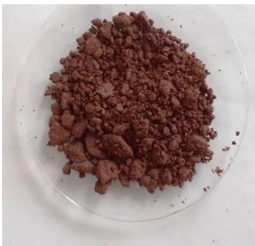
Figure 3. Petroleum contaminated soil sample
