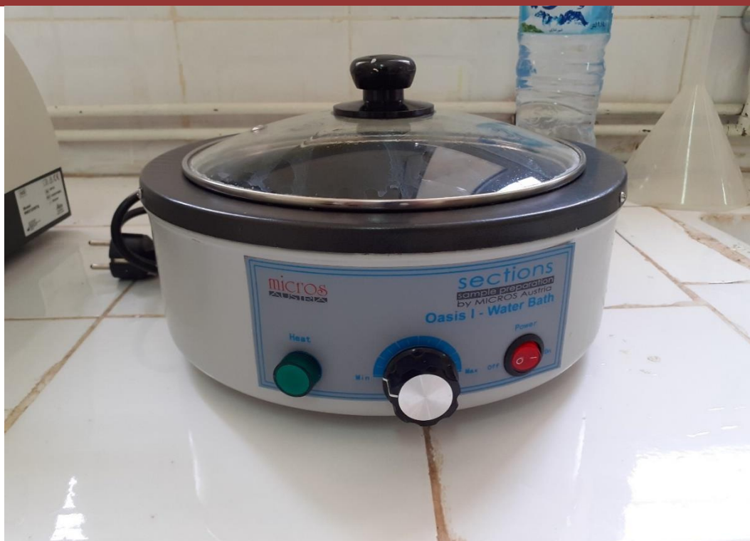
Figure 32 : Bain marée (Oasis 1 water bath)
