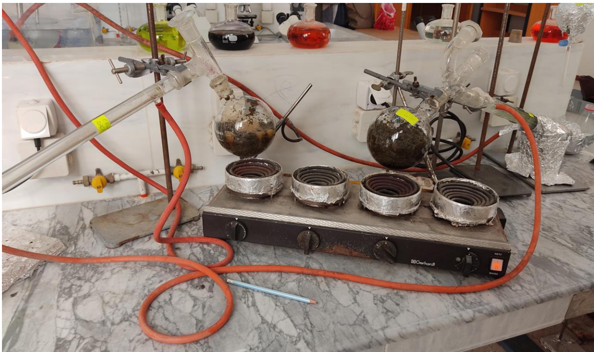
Figure 28 : Montage d'hydro distillation (Photo originale)
