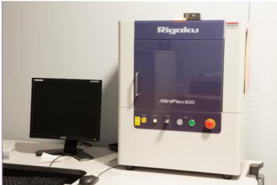
**Figure III.5:** Diffractomètre Rigaku miniflex 600 X-ray.
