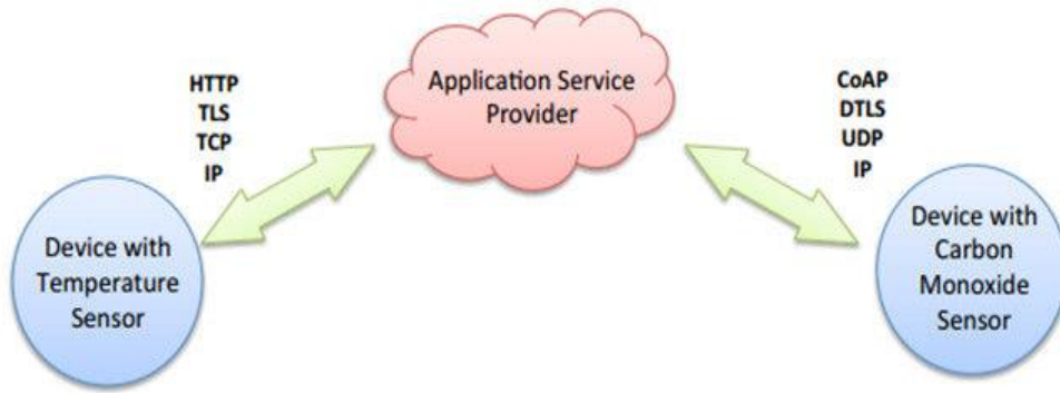
Figure 3:device to cloud communication model [3]
