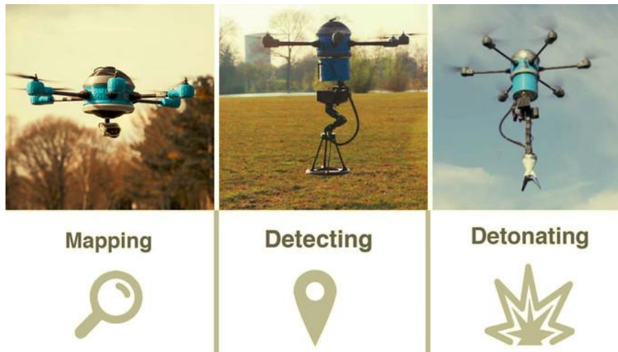
Figure 11: A drone that can maps, detect and detonate landmines
