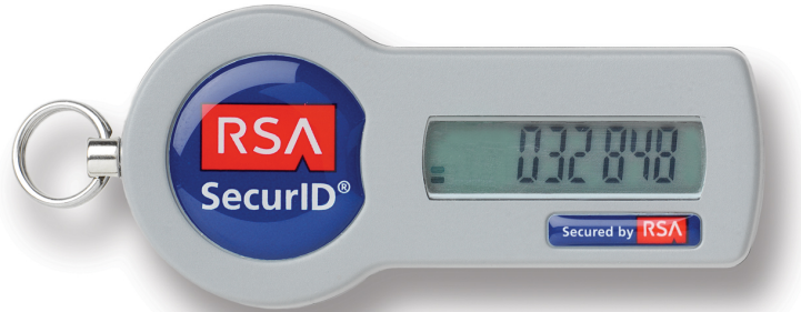
Figure 1.3: The RSA SecurID hardware token generates a new code every 30 seconds [13]
