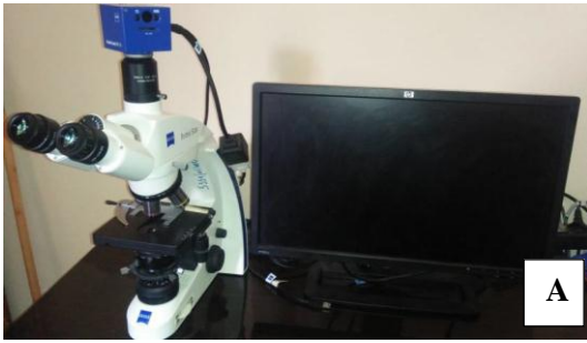
Microscope ZEISS PrimoStar muni d'une camera AxioCamEPC.
