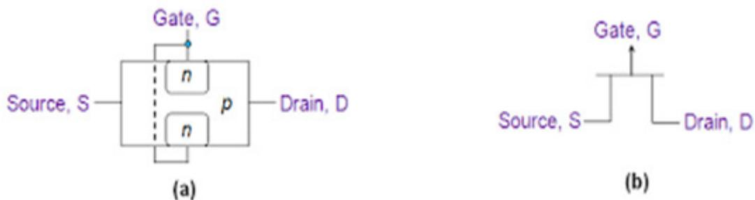
Figure 4.10. NPN Junction Field Effect Transistor.
