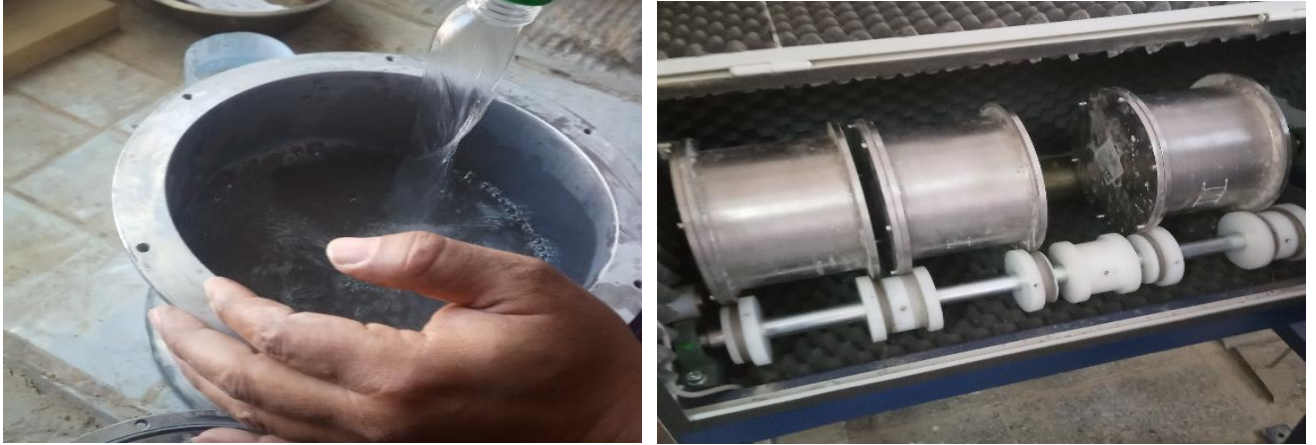
Figure (III. 6) Essai Micro-Deval
