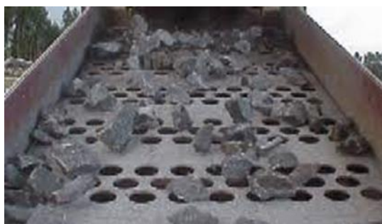
Figure (II. 16) criblage des granulats
