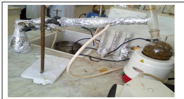
Figure 4 : Montage d'hydro-distillation (Originale)
