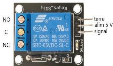
Figure 3.12 : Module relais 5V-220V [35]
