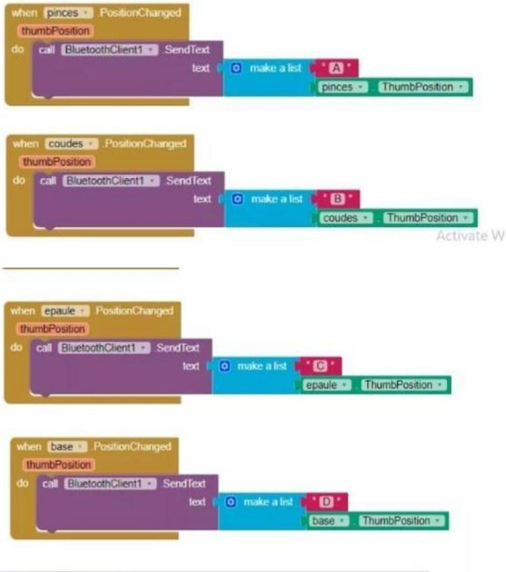
**Figure VI.8 :** Les blocs de programmation application via Bluetooth
