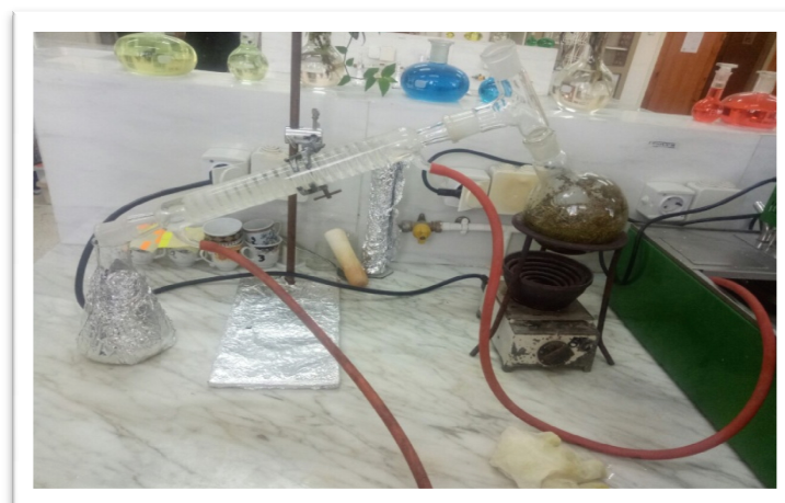
Figure 4 : Le Montage de distillation (Original)
