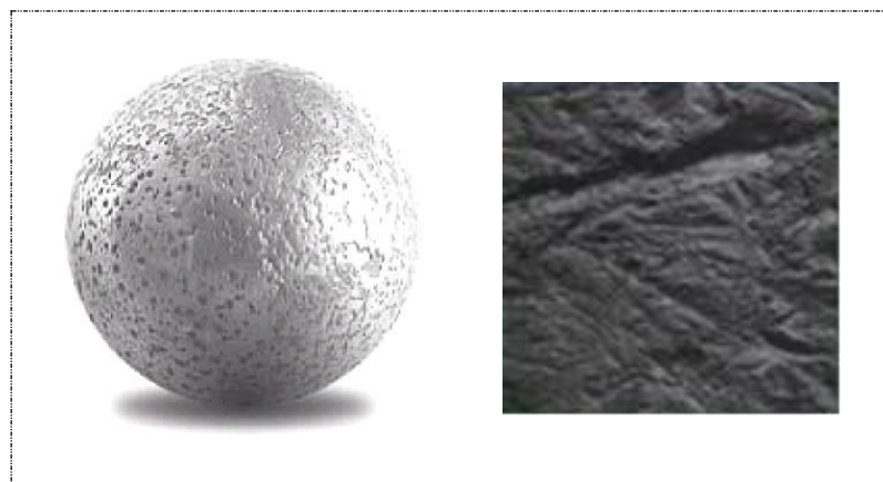
Figure II. 10. Usure abrasive des boulets de broyage
