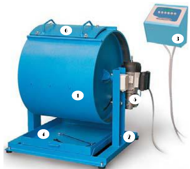
Figure III.1. Machine d'abrasion "Los Angeles" [32]
