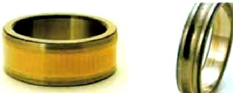
Figure III.12 : Corrosion de contact.
