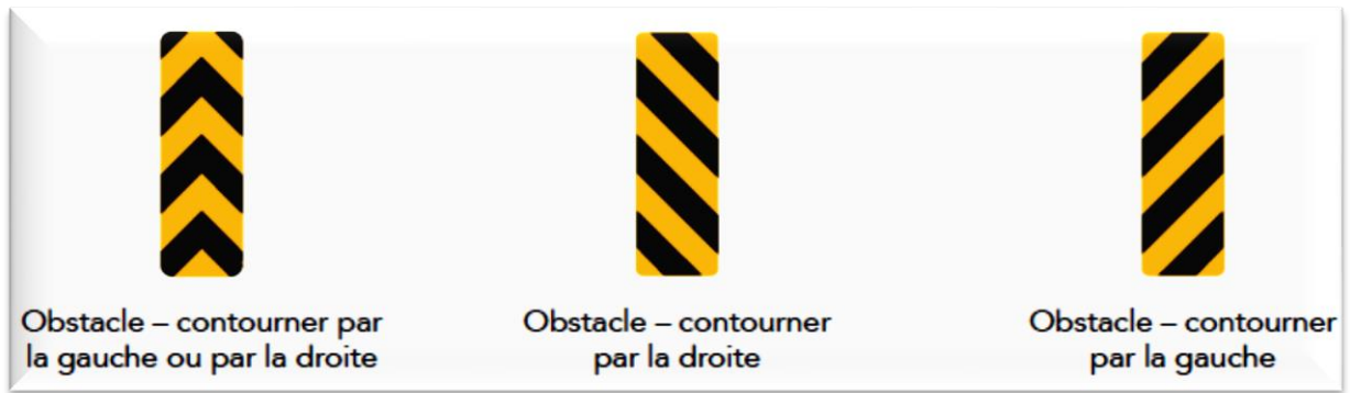
Figure XII- 6: Balises de danger.
