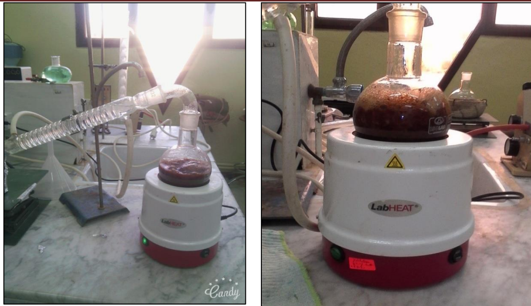
Figure 5: Montage d'hydrodistillation (clevenger 1928)
