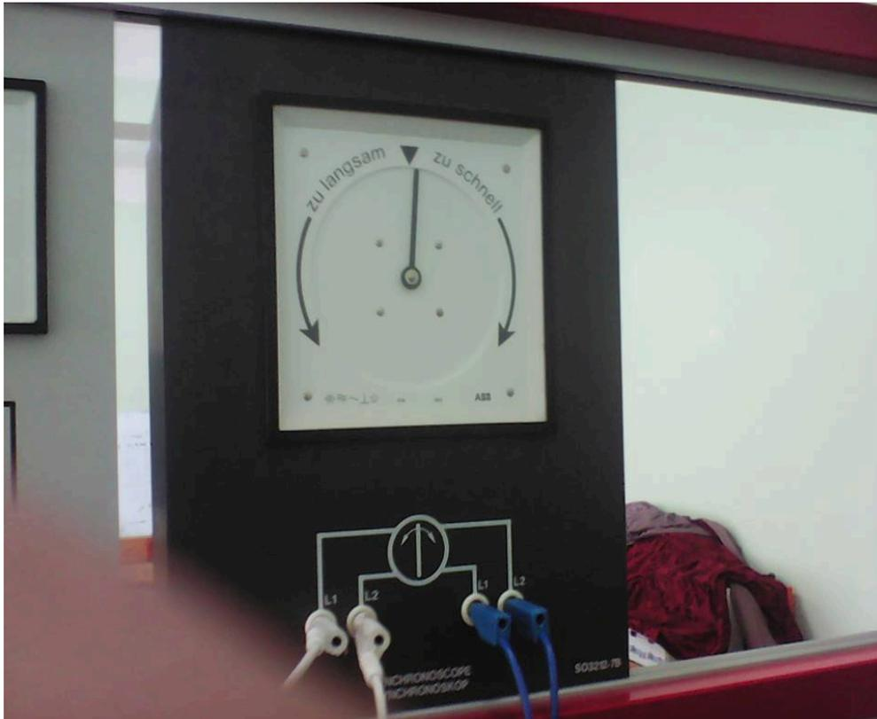
Fig.IV.20 : synchronoscope
