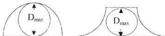
**FIGURE 2-11: DIAMETRE MAXIMUM ADOPTE A LA SECTION DE PASSAGE**
