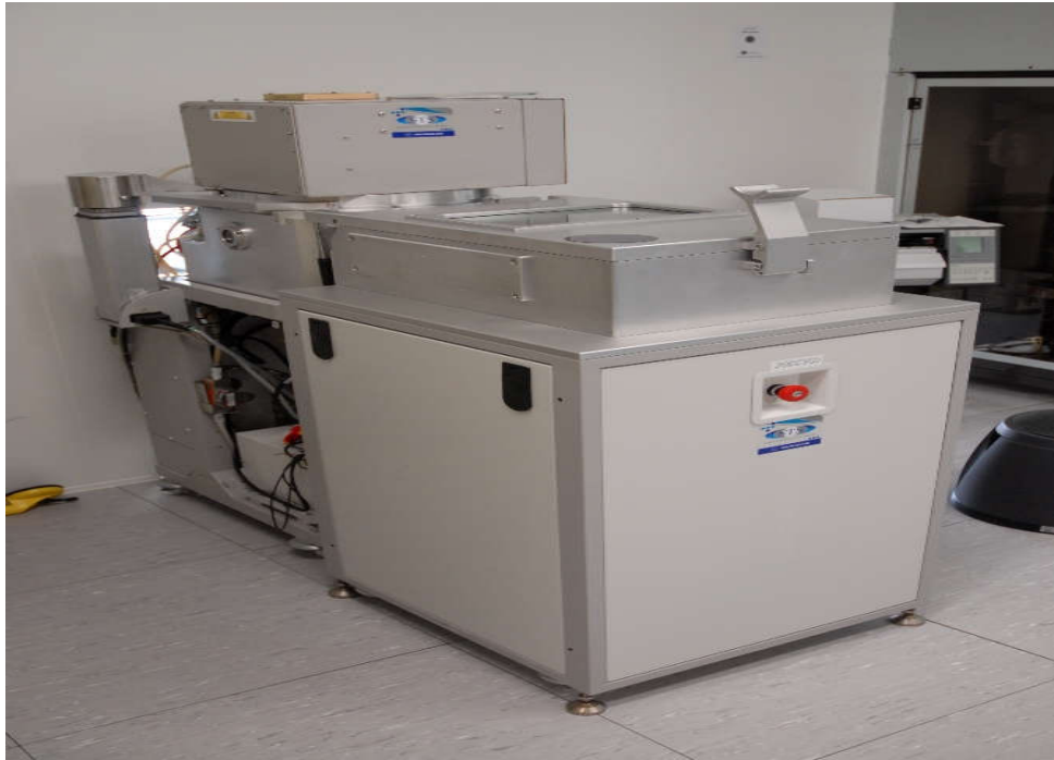
Figure 1.9 PECVD (Plasma-enhanced chemical vapor deposition) machine.
