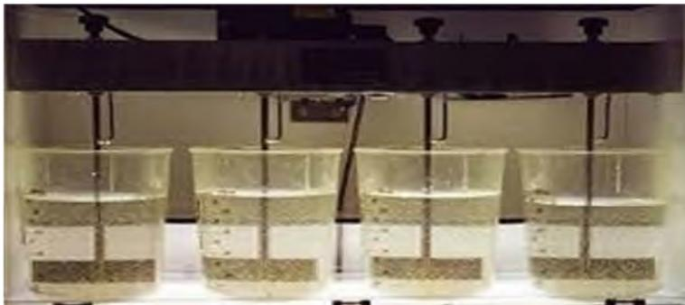
**Figure I.2: Coagulation-floculation**
