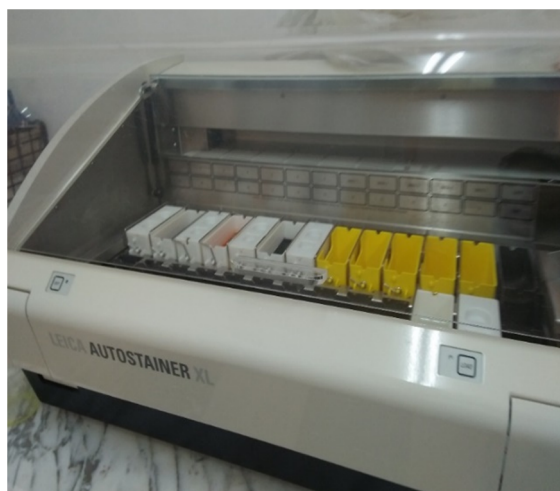
Figure 2. Automate de coloration Papanicolaou (Leica Autostainer XL).
