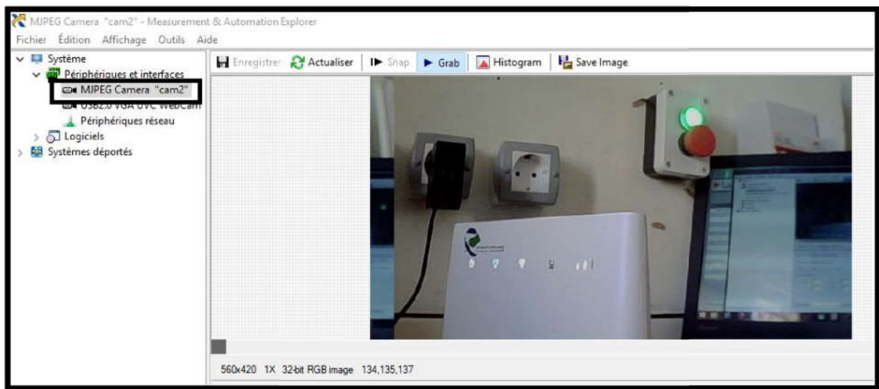
Figure II. 10 Test de la camera sous LABVIEW (NI MAX)
