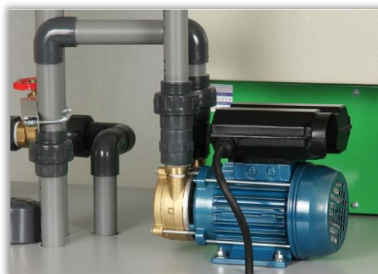
Figure II.13 la pompe de surface
