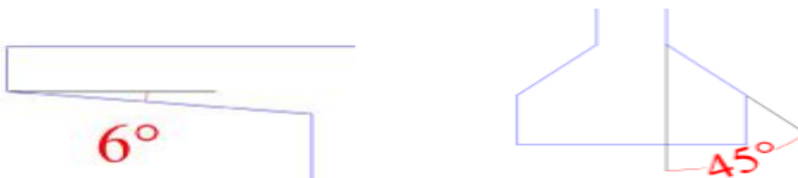
Figure I.4: Angle des goussets
