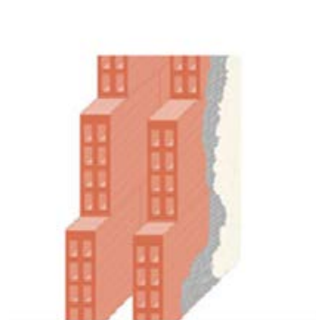
Mur double cloison
