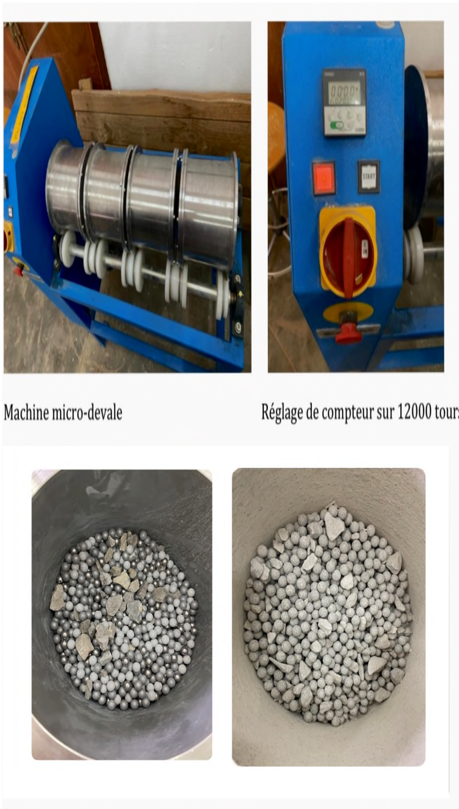
Figure .IV.15. Essai Micro- DEval
