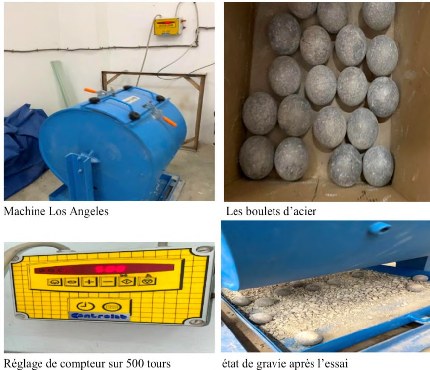
Figure .IV.14. Essai Los Angeles
