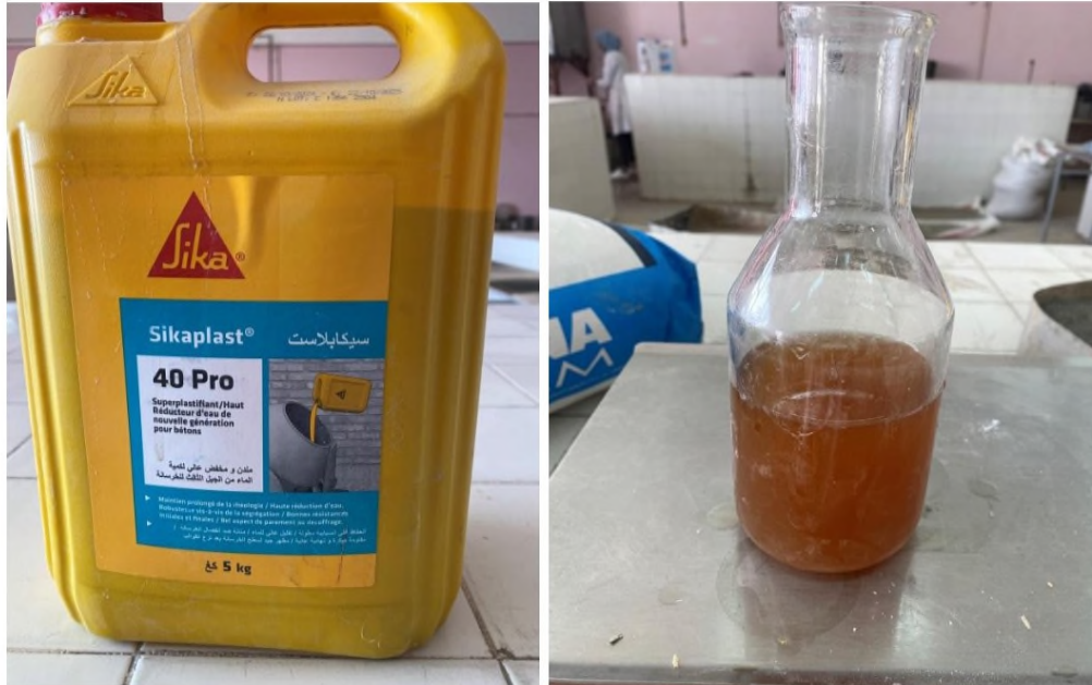
Figure .IV.6. Adjuvant superplastifiant SikaPlast-40 Pro.
