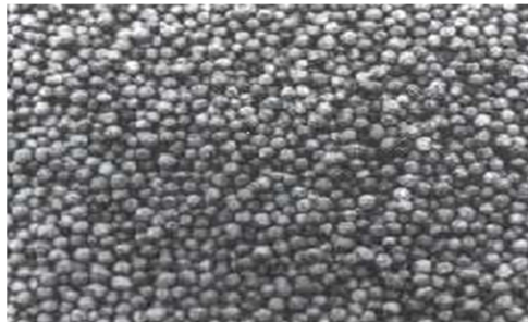
Figure III.2 : Structure non consolidée.
