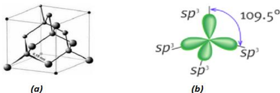
Figure I.7: a) Structure cristalline b) Orbitales hybrides sp^3 de carbone de diamant
