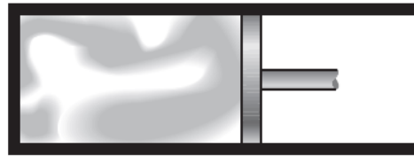
b) Quasi-equilibrium expansion and compression of a gas
