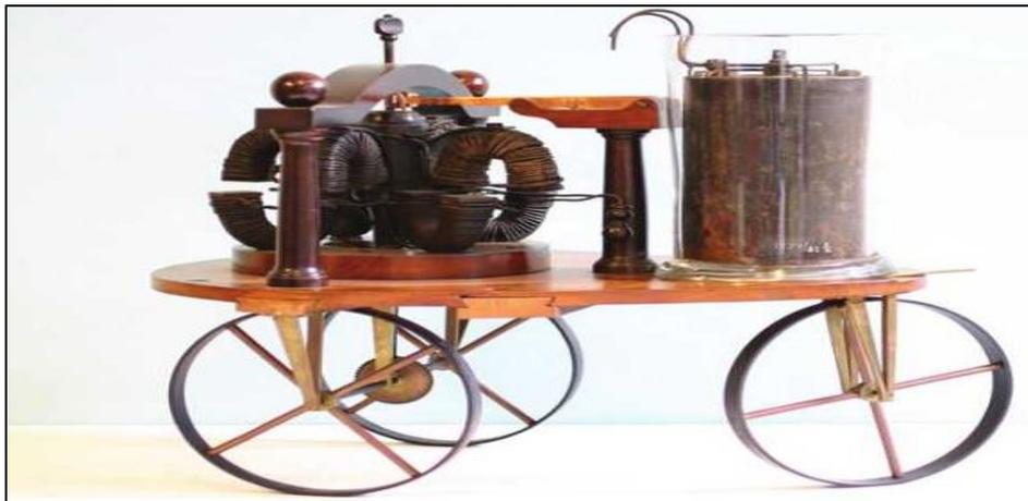
**Figure I.2.** Sibrandus Stratingh 's electric horseless carriage [85].
