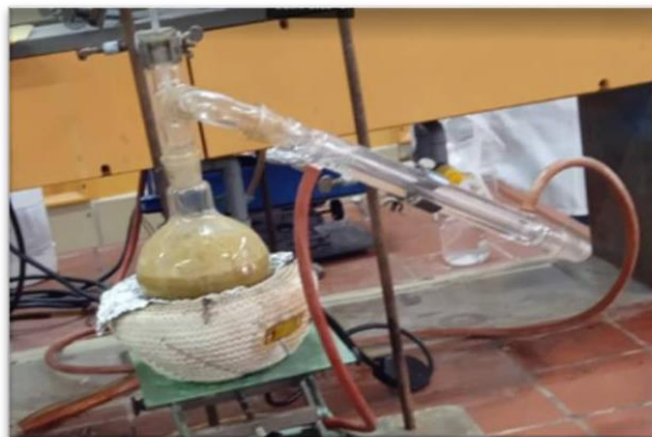
Figure II.6: The hydrodistillation experience.
