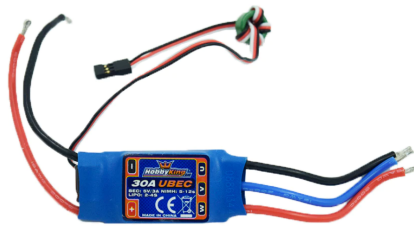
Figure 1.14: The electronic speed variator (ESC)[22]
