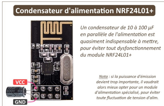
Figure 1.10: The power capacitor with the NRF24L01+ module[20]
