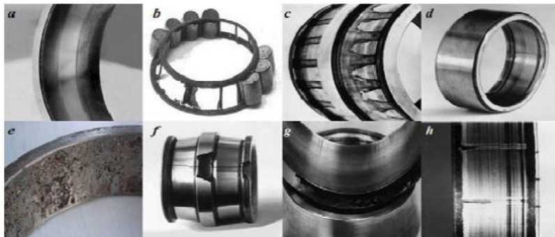
Figure II.11 — Some failures affecting the bearings: a- Generalized wear b- Deteriorated cage c- Corrosion d- Presence of craters e- Flaking f- Cracking and breakage g- Seizure h- Trace marks [27].
