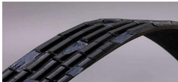
Figure II.12 — Belt Fault (Pull-Out) [26].
