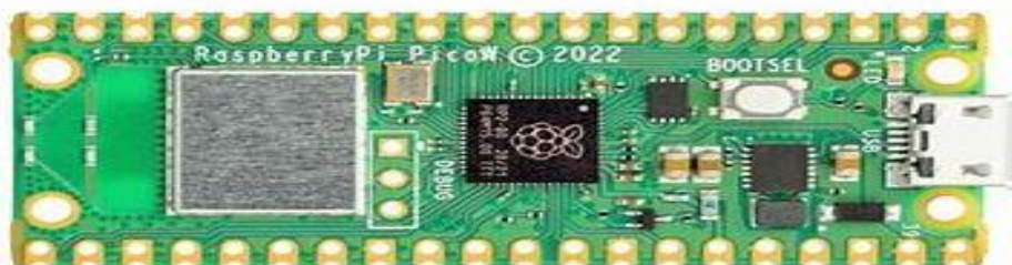
Figure III. 17: rpi pi pico w
