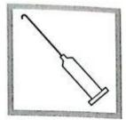
Insert a clean delivery tube into the digital titration cartridge. Attach the cartridge to the Digital Titrator.
