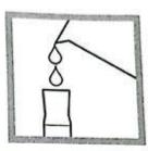
Use a graduated cylinder or a pipet<sup>1</sup> to measure the sample volume from Table 1 on page 3.
