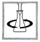
13. Put the end of the delivery tube fully into the solution. Swirl the flask. Turn the knob on the Digital. Titrator to add titrant to the solution. Continue to swirl the flask. Add titrant until the color changes from red to yellow. Record the number of digits on the counter.
