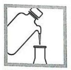
If the sample volume is less than 50 mL, dilute to approximately 50 mL with deionized water.
