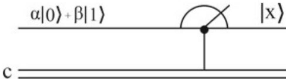
Figure 15: Measurement of a single qubit [10]
