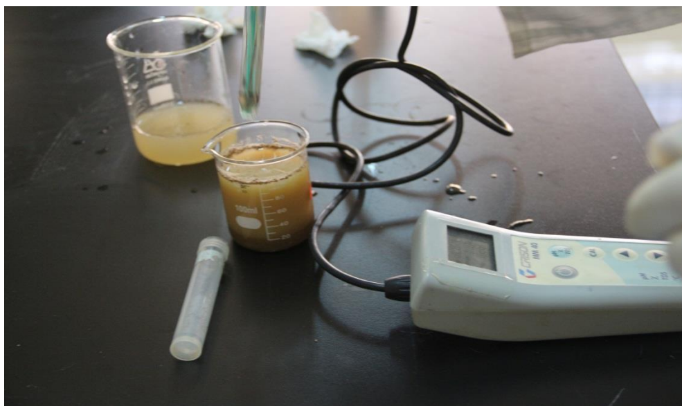
Figure 35: Measurement of the electrical conductivity of the ground by the conductivity meter
