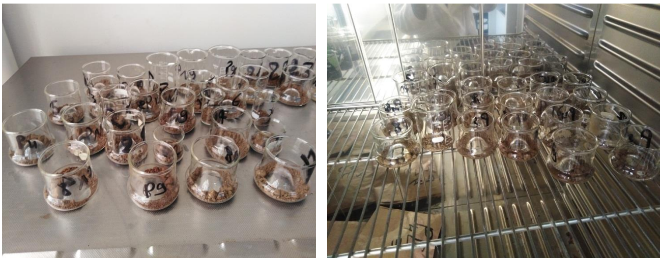
Figure 31: Weighed and oven-dried soil samples (Cliche SENOUCI SOUAD, 2023)
