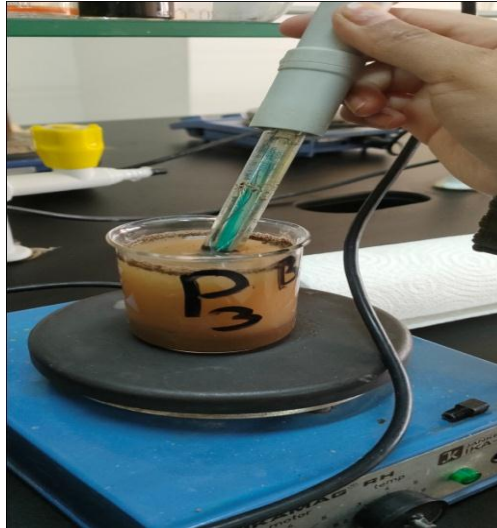
Photo 5: Measurement of soil electrical conductivity using a conductivity meter. (Cliche Tlidji).
