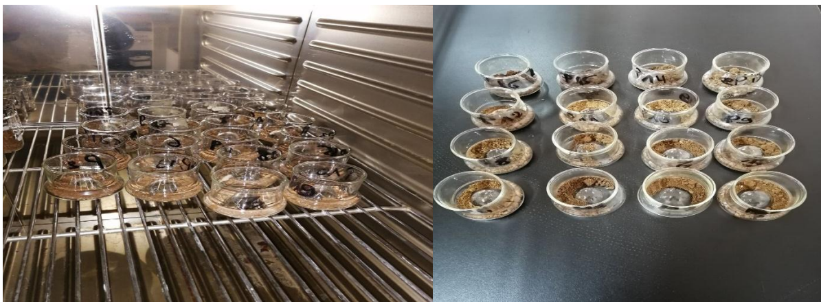
Photo 2: Weighed and oven-dried soil samples (Cliche Benouadah).
