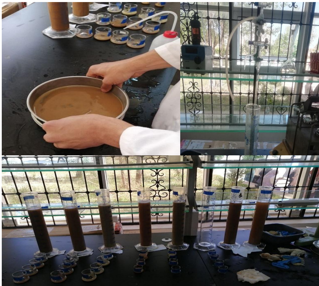
Photo 3: Granulometric analysis using the Robinson pipette method (cliche Benouadah).
