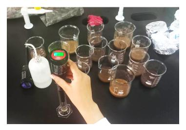
Figure 22: NPK Measurements (S.Saadna)
