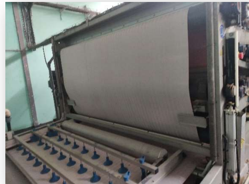
Figure 16: the perforated belt filter and the press filter for (Original photo)
